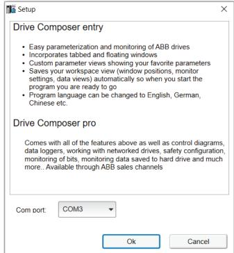
Choose the COM port your cable is connected to. (If it is the only usb device you have connected, it is the only one displayed)
