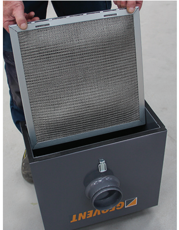
7. Insert the new filter. Gently fit it into the frame. Push it all the way to the bottom of the filter box.
