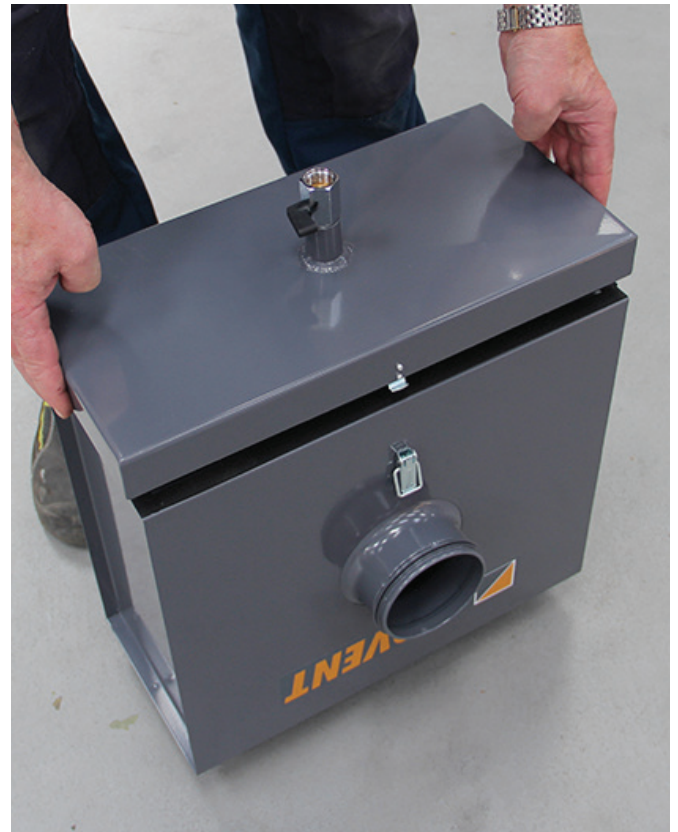
8. Gently push the filter into place. It may be necessary to lift the filter up a littel to make it fit. Afterwords the lid is placed on the filter box and lucked.
