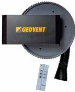
Electric hose reel with wireless remote control. ø160 mm nipple and 1x 230V. With hose but without nozzle.
